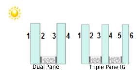
In triple-pane constructions where LoĒ -i89® (#6) is used, LoE-180® is recommend for the center pane: see Cardinal's TSB IG07 Heat Treatment recommendations. The location of the coatings in a triple-pane has minimal effect on performance.
