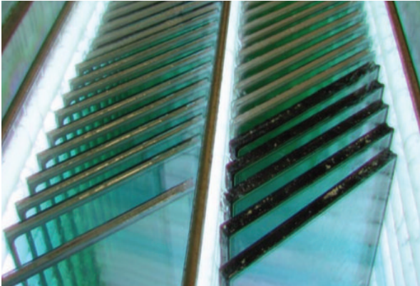
P-1 Test Chamber: 140°F, constant UV, 100% humidity
