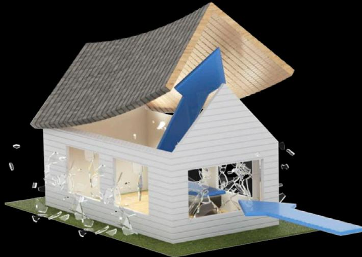
When a building is breached through a broken window, wind can enter the building and create a sudden pressure increase that lifts the roof and pushes the walls outward, causing the building to collapse.
