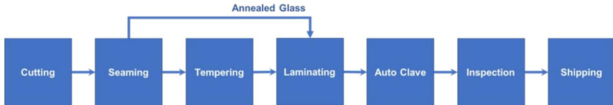
**Figure 1:** Laminating process diagram
