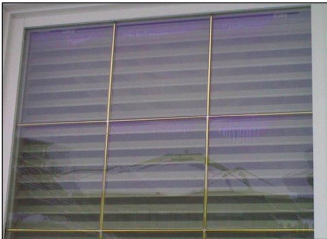
Fig. 10-1: Chemical fogging as seen in a non-Cardinal IG produced unit. Chemical can be seen running down glass in area of internal grilles
