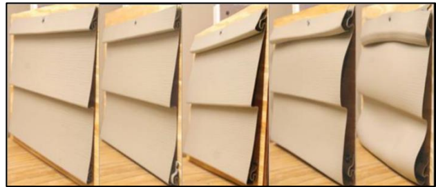
Not heated (A) 160 °F (B) 165 °F (C) 170 °F (D) 180 °F Figure 3. Vinyl Siding Heated for One Hour
